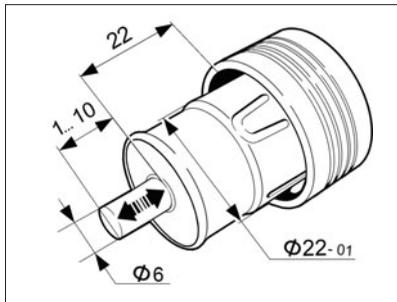
**Fig. 21c. Electrical device plug
