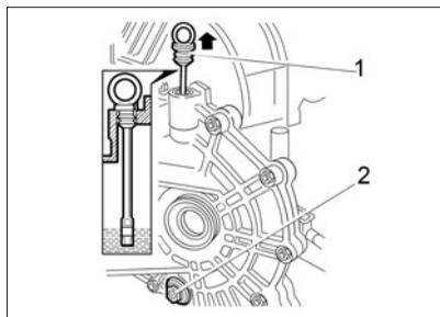
**Fig. 46a. Gearbox oil level checking**
