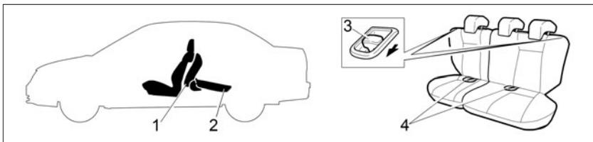
**Fig. 11b. Folding down the rear seat with the headrests
