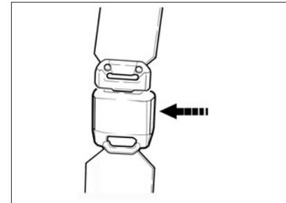
Fig. 14c. Mini-lock of the back middle seat passenger seat belt
