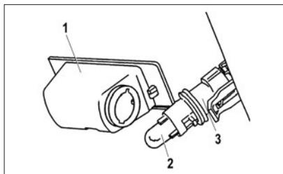
**Fig. 61b. Licence plate light in «liftback» vehicle**
