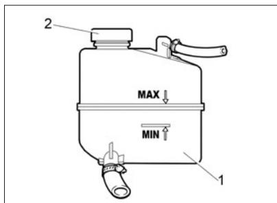
**Fig. 49. Expansion chamber**
