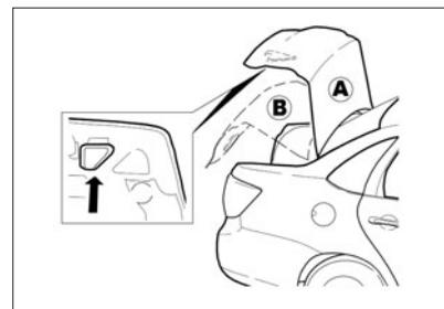
**Fig. 26b. Trunk lid inside handle (in the design variant)**
