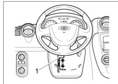
**Fig. 12. Steering wheel position adjustment
