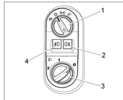
**Fig. 32a. Lighting engineering control module and dipped beam adjuster**
