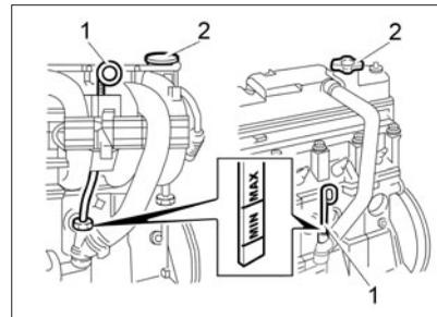
**Fig. 45. Engine case oil level checking**
