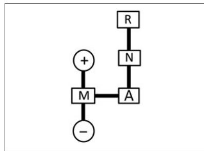
Fig. 48. Gear change lever scheme
