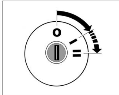
**Fig. 36. Ignition starter switch**
