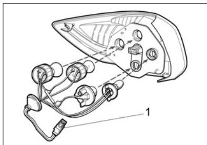
**Fig. 60b. Rear light in «liftback» vehicle**
