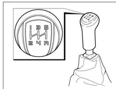
Fig. 37b. Gear change lever in mechanical transmission (in the design variant)
