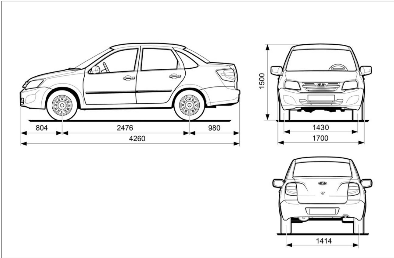
**Fig. 66. Overall (reference) dimensions of the vehicle 2190 («sedan»)**
