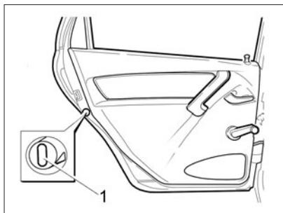
Fig. 8. Latch hook spline
