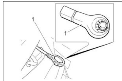
**Fig. 33. Rain and light sensor**
