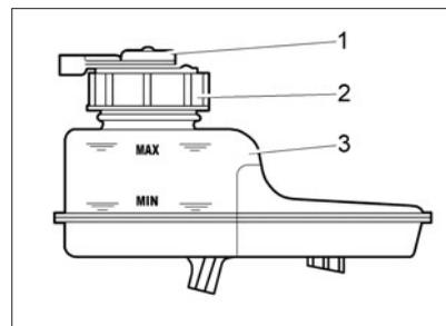
**Fig. 50. Hydraulic brake actuation fluid reservoir**
