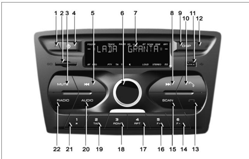
**Fig. 2. Control panel of radio (optional design)**
