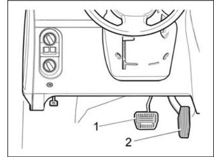
Fig. 37d. Pedals with automatic transmission
