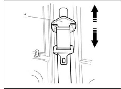
Fig. 14b. Adjusting the seat belt
