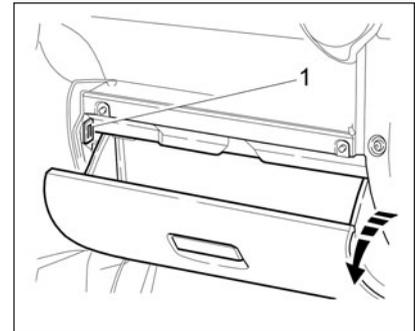
Fig. 41c. USB connector location
