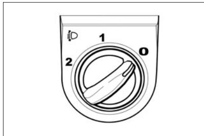
**Fig. 32b. Dipped beam headlights adjuster**
