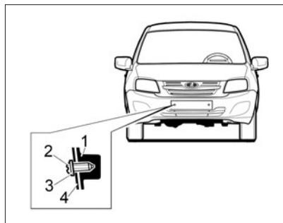
Fig. 42a. Fastening of number plates
