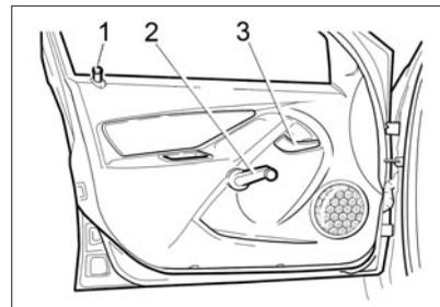
Fig. 4b. Left hand front door with the speaker
